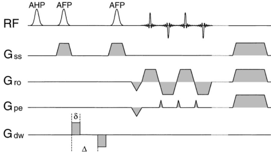
where  $\gamma$  is the gyromagnetic ratio of a proton,  $G$  is a bipolar gradient strength,  $\Delta$  is the intergradient separation, and  $\delta$  is the gradient duration. Typical values for the parameters used in this work were  $\Delta = 10$  msec, and  $\delta = 5$ – $8$  msec. Various  $b$  values up to  $1200$  sec/mm<sup>2</sup> were achieved by adjusting the gradient strength up to  $30$  gauss/cm.
